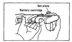
Do not use force when inserting the battery cartridge.
